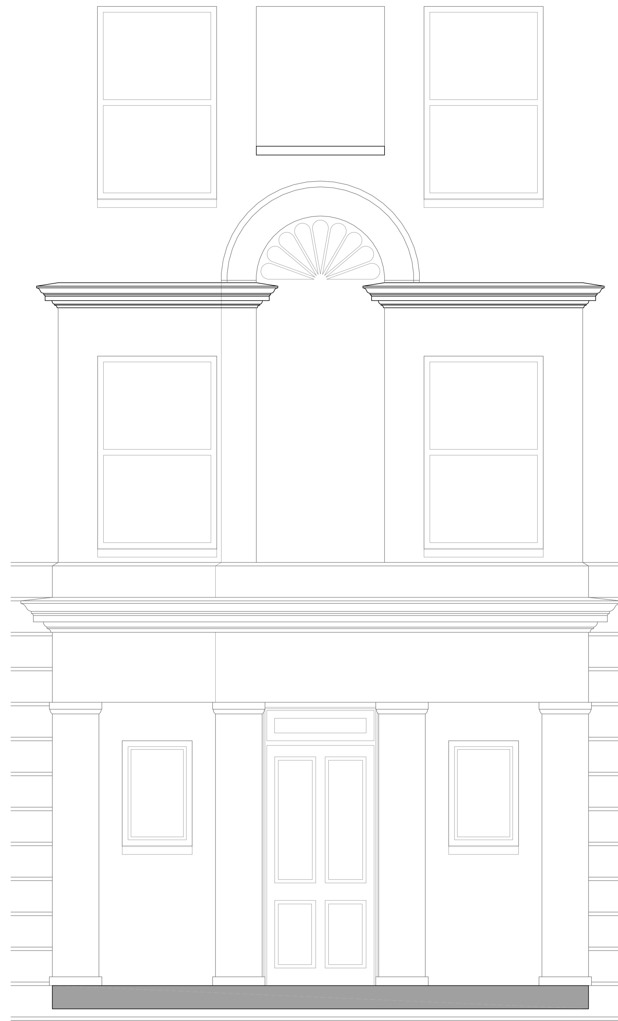
Door Casing - Elevation
