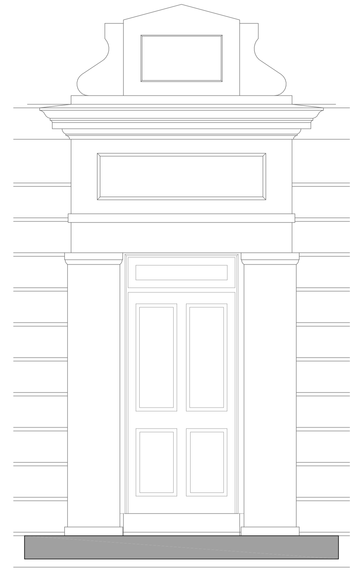
Door Casing - Elevation
